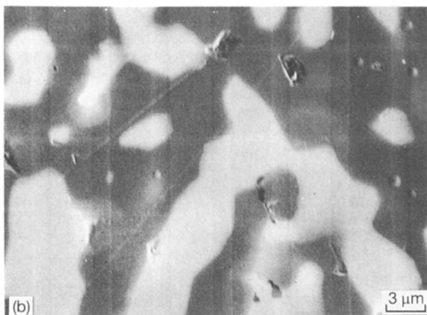
Figure 2 SEM micrographs of 30 vol % \text{Cr}_3\text{C}_2 (1.5 \mu\text{m} particle size) reinforced \text{Al}_2\text{O}_3 matrix composites hot-pressed at (a) 1400, (b) 1700 °C. White particles are \text{Cr}_3\text{C}_2 distributed in grey \text{Al}_2\text{O}_3 matrix.
